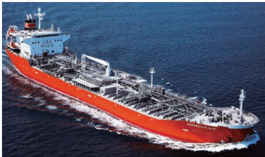
M/T "CHEMROUTE SUN" 25,615.00DWT L.O.A:159.03m Breadth:27.10m Depth:14.20m Build : Mar/2008 Shin Kurushima Hiroshima Dockyard Co.,Ltd.
